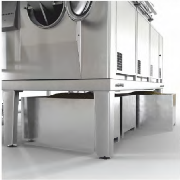
← Unloading into several mobile stainless steel containers
