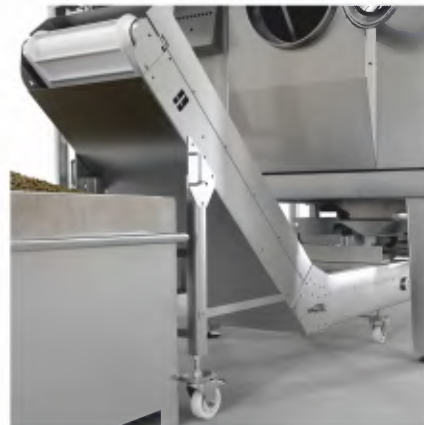
← Unloading into several mobile stainless steel containers
