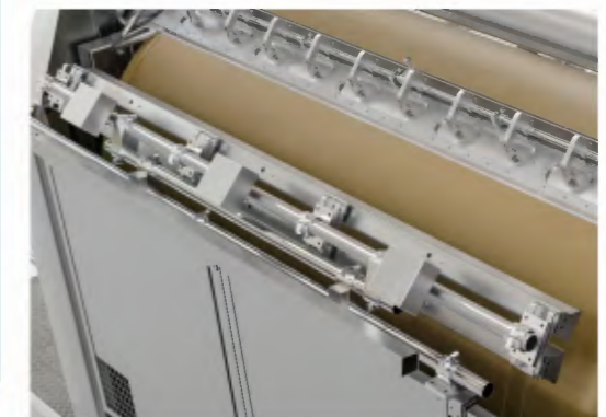
IR drum heating to prevent the chocolate from sticking to the drum wall
