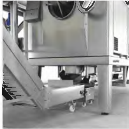
Unloading by vibration chute mounted underneath the unloading hopper
