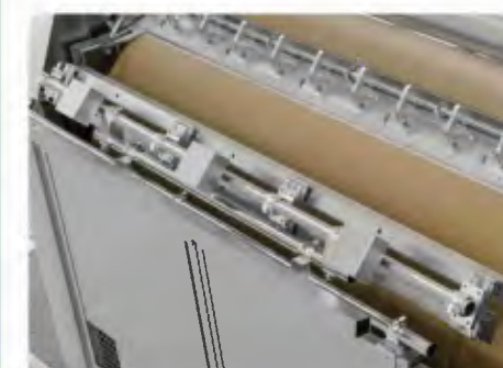
IR drum heating to prevent the chocolate from sticking to the drum wall
