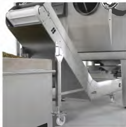
Unloading by flat belt and ascending belt
