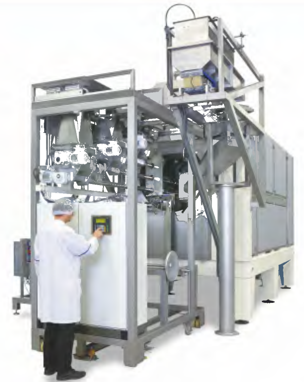
The DRIACONTI-T continuous coater gains efficiency by reducing labor as well as overall manufacturing costs
