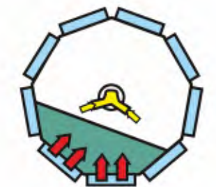
Reverse axial flow from the bottom of the drum through the product to the hollow shaft
