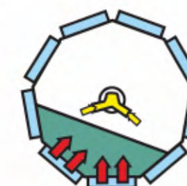
Reverse axial flow from the bottom of the drum through the product to the hollow shaft
